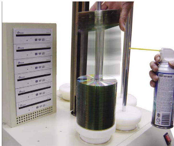
Figure 1-1 Using Canned Air to Reduce Static
