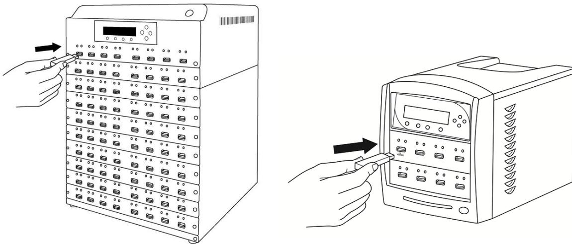
Step 5. Insert empty target flash devices (ex. USB, SD, CF, etc) (the drive(s) to receive data) into the other non-Source ports.
