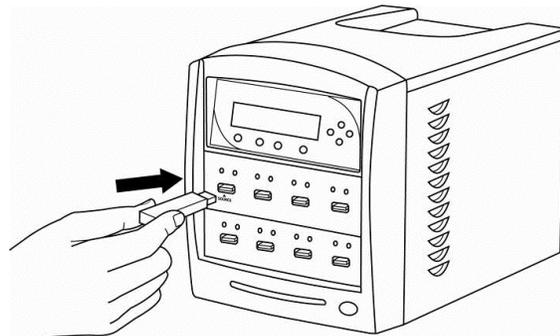
Step 4. Insert empty target flash devices (ex. USB, SD, CF, etc) (the drive(s) to receive data) into the other **non-Source** ports.
