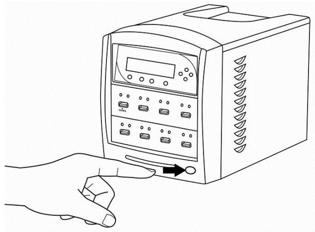
Step 2. After it has booted up, the screen on the left should appear signifying the system is ready. Press the “F1 Smart Copy” button to initiate the copying process.
