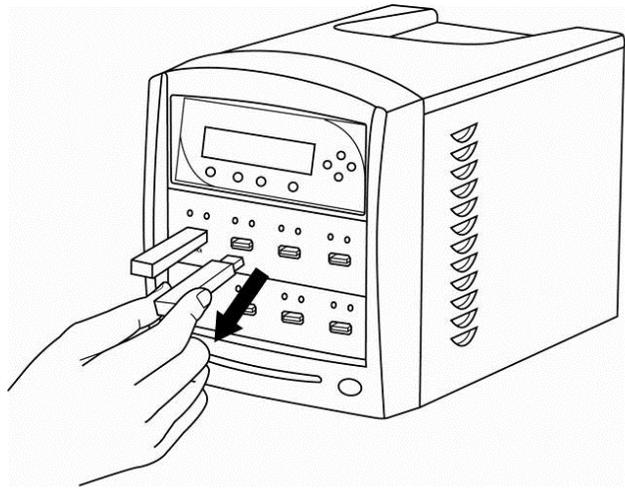
Make more copies by connecting more flash devices (if so, return to step 3) or end the job and go back to the root menu by pressing the “ESC” button.
