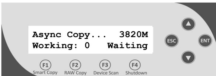
The job can be ended immediately and the unit returned to the root menu by pressing the “ESC” button.
