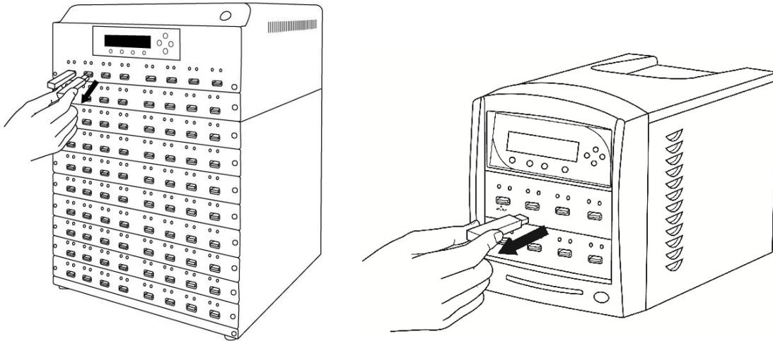
If additional flash devices are to be copied, the new devices can be added without waiting for all the others to completely finished. The new ones can be inserted on the fly.
